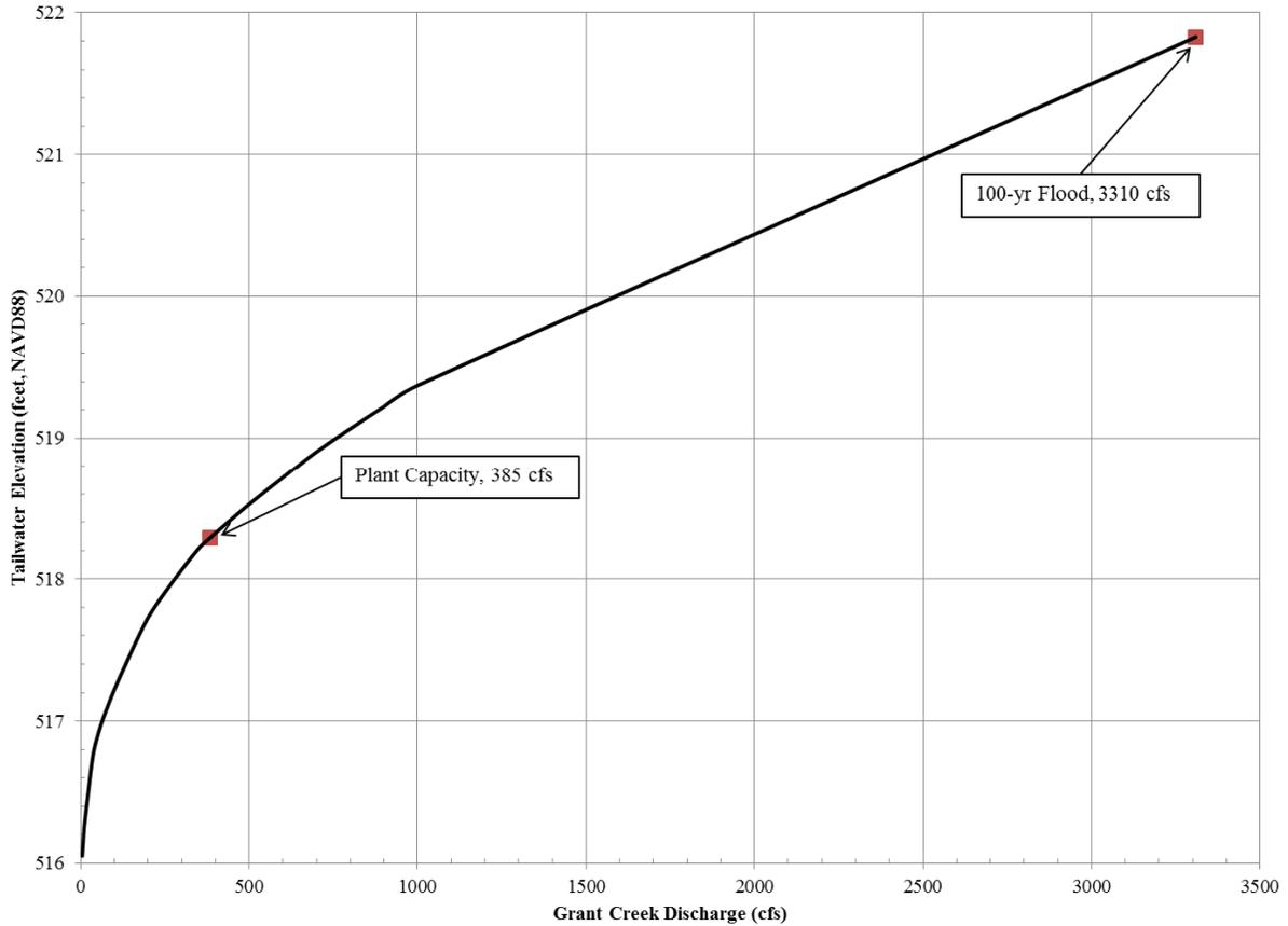
**Figure B.3-7.** Grant Lake tailwater rating curve.
