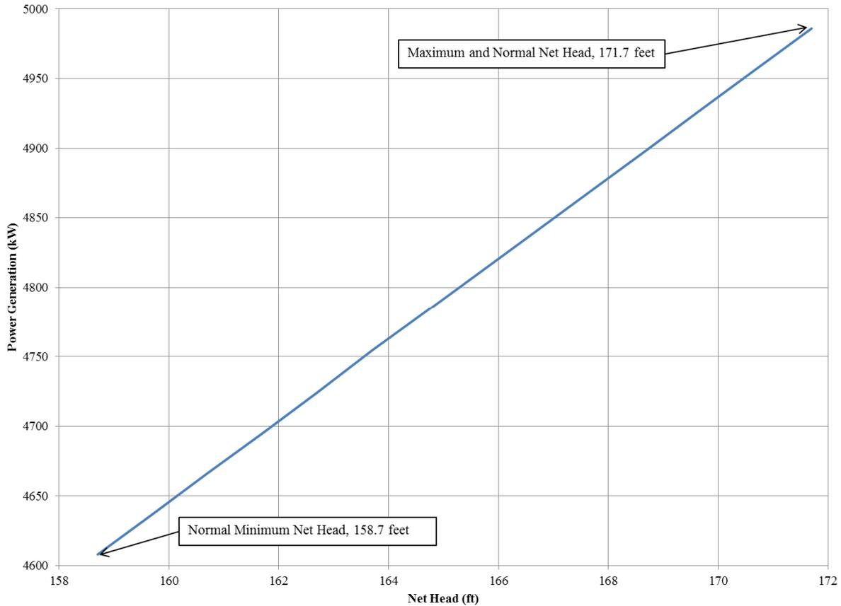
**Figure B.3-8.** Project power generation vs. net head.
