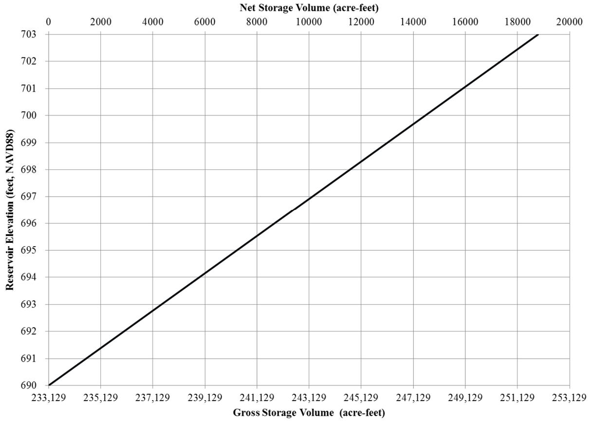
Figure B.3-4. Grant Lake storage capacity curve.
