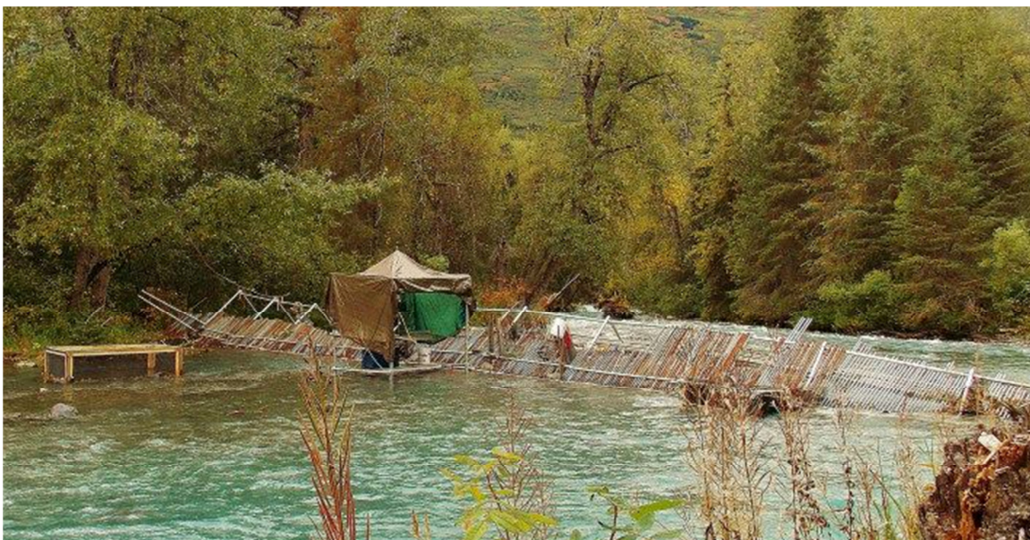
Figure 4.1-1. The A-frame weir used on Grant Creek to count adult salmon, rainbow trout and Dolly Varden in 2013.
