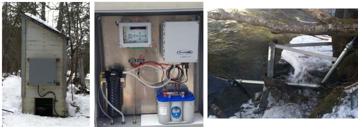
Figure 4.1-1. GC 200 enclosure, data logger, bubbler line, and staff gage installation.
