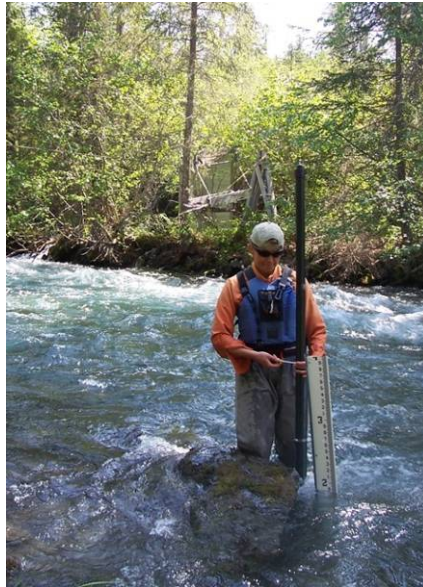
Figure 3. Example staff gage and data logger installation.
